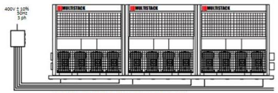
Electrical box and related wiring (not supplied by manufacturer)
