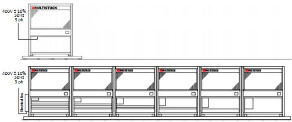
Electrical box and related wiring (not supplied by manufacturer)
