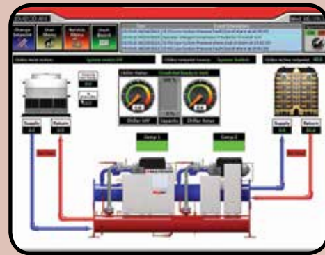
Example of a typical Home Screen with chiller graphics.
